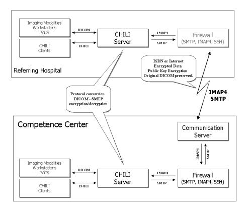
Figure 2. Protocols between the components
